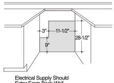
Electrical Supply Should Enter From Back Wall In Shaded Area.
