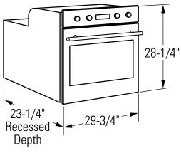
**Side by Side Installations** Install two wall ovens in separate cutouts. Allow 2" (5.1 cm) min. between cutouts.
