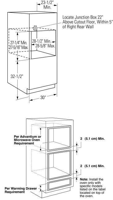
The solid bottom or runners must be level with the bottom of the cutout, or the bottom trim may not install correctly and could interfere with the door opening. If the cabinet does not have a solid bottom, two braces or runners must be installed level with the bottom of the cutout to support the weight of the oven. The runners and braces must support 200 lbs. (90 kg).
