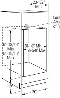
Locate Junction Box 47" Above Cutout Floor, Within 5" of Right Rear Wall
