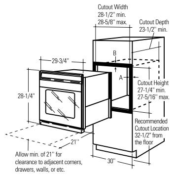
A = Allow 11/16" - 3/4" for overlap of oven over side edges of cutout. B = Allow 1" overlap of oven over top and 1-1/4" overlap at the bottom edges of cutout.
