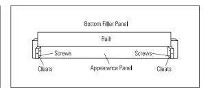
**Note:** The screws should be long enough to secure rail to the filler panel without penetrating the finished face of the filler panel.
