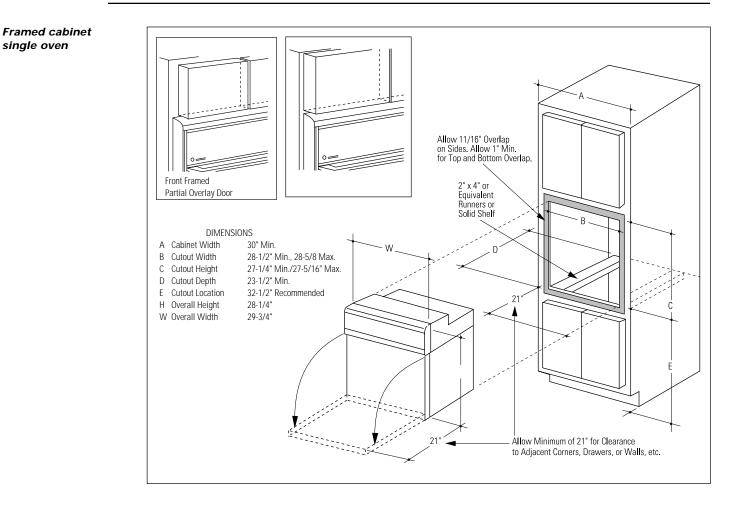
Use the information in this dimension drawing for typical framed cabinets. The front face of the oven will be flush with cabinetry doors or drawers.
