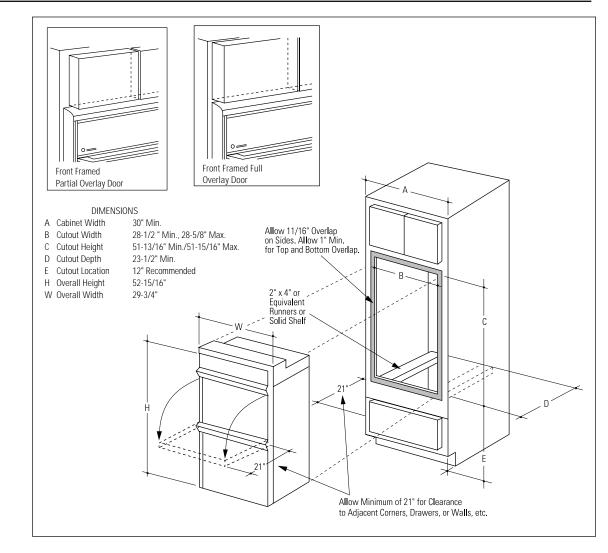
Use the information in this dimension drawing for typical framed cabinets. The front face of the oven will be flush with cabinetry doors or drawers.
