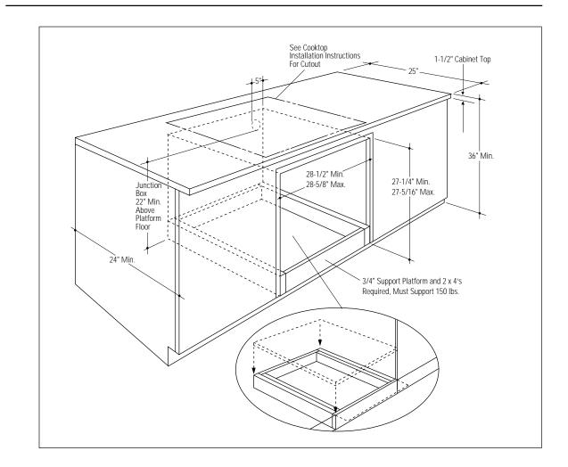
These ovens can be installed below a countertop. The rough opening of the base cabinet should be:
