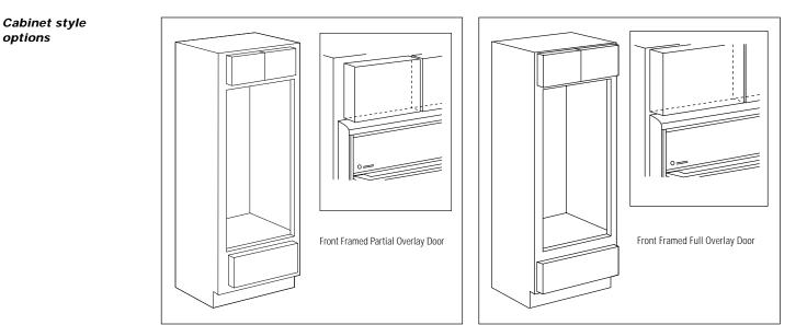
Monogram ovens are installed directly into a wall or wall oven cabinetry, 30" minimum width. The front surface of the ovens will be nearly flush with surrounding cabinetry. To obtain optimal appearance, cabinet cutouts must be exact. The examples shown here illustrate typical styles of 30" cabinets and oven fit. Installation instructions for each of these basic cabinetry styles are provided in this section.
