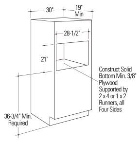
Order a 30" wide single oven cabinet or cut the opening in a wall to dimensions shown.
