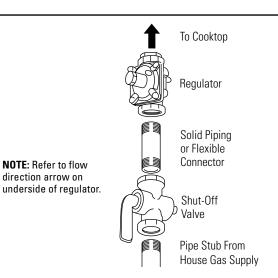
**IMPORTANT:** Disconnect the cooktop and the individual shut-off valve from the gas supply piping system during any pressure testing of that system at test pressures greater than 1/2 psig. Isolate the cooktop from the gas supply piping system by closing the individual manual shut-off valve to the cooktop during any pressure testing of the gas supply piping system at test pressures equal to or less than 1/2 psig.
