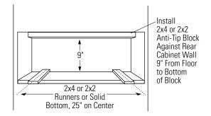
**NOTE:** The support must be level, rigidly mounted and capable of supporting 150 lbs.
