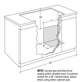
• A properly-grounded 3-prong receptacle should be located within reach of cooktop's four foot power cord.
