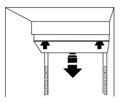
To reinstall the upper fresh food shield, hook the front edge first, then push it up and back until the shield rests in place.
