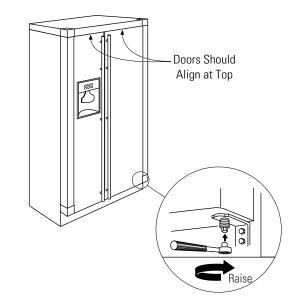
**NOTE:** A nylon plug is imbedded in the threads of the pin. The plug is designed to prevent the pin from turning. A wrench must be used to turn the pin.
