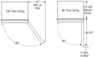
Allow 25" minimum clearances for a full 130° door swing. Allow 15" for pan removal.
