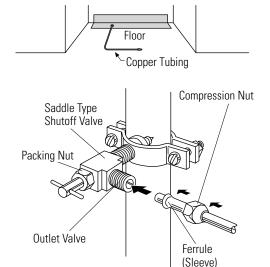
**NOTE:** It is best to install the valve into a vertical water pipe. If you install the valve into a horizontal water pipe, make the connection at the top or side to avoid drawing off any sediment from the water pipe.
