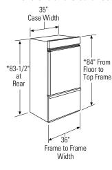
\* Shipping height. The refrigerator can be adjusted to fit into a cutout that is 83-1/2" min. to 84-1/2" max. height. Note that the top case trim at the front is 1/2" higher and will overlap upper cabinetry or soffit. Use leveling legs and wheels for height adjustment.
