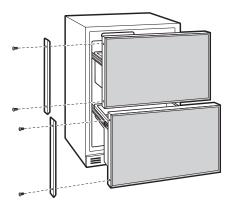
**6.** Place the brushed decorative covers over the side trim to hide the screw heads. Ensure side trim is aligned top-to-bottom and front-to-back. Snap into place.
