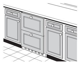
Cut-out dimensions: Height:  $34^{1/2''}$  (876 mm) minimum Width:  $23^{3/4''}$  (603 mm) minimum Depth: 24'' (610 mm)
