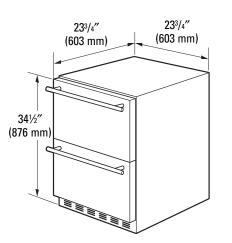
Product dimensions:Height:  $34^{1/2}''$  (876 mm)Width:  $23^{3/4}''$  (603 mm)Depth:  $23^{3/4}''$  (603 mm)
