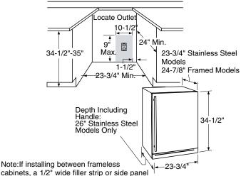
cabinets, a 1/2" wide filler strip or side panel may be required. The filler strip will act as a spacer between the door case and adjacent cabinet and will prevent interference with cabinet door swing. The width of the opening must include filler panels.
