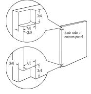
Assemble overlay panels with glue and screws.
