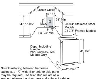
cabinets, a 1/2" wide filler strip or side panel may be required. The filler strip will act as a spacer between the door case and adjacent cabinet and will prevent interference with cabinet door swing. The width of the opening must include filler panels.
