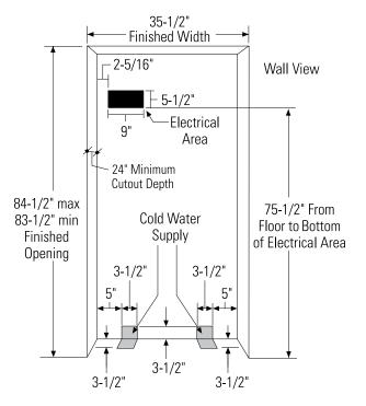
The water and electrical supply must be located as shown. The finished cutout width must be 35-1/2". **Note:** The case trim overlaps cabinets at the top and sides. Frameless cabinets may require filler strips to prevent interference with cabinet door swing. The opening width must allow for filler strips.
