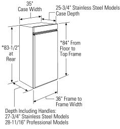
\*Shipping height. The refrigerator can be adjusted to fit into a cutout 83-1/2" min. to 84-1/2" max. height. Note: the top case trim at the front is 1/2" higher and will overlap upper cabinetry or soffit. Use leveling legs and wheels for a maximum 1" height adjustment.
