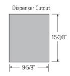
\*Cut the dispenser opening after the backer, spacer and overlay panels have been assembled.
