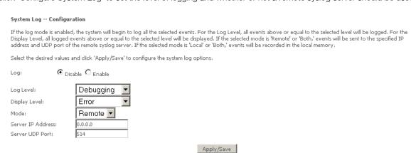
If a remote system log server is to be used, enter the IP address and port the remote syslog server is running on.
