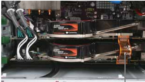
SLI bridge cable
