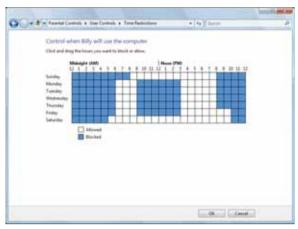
3 Click inside the grid to set when the user can access the computer. Blocked hours are blue, and allowed hours are white.
