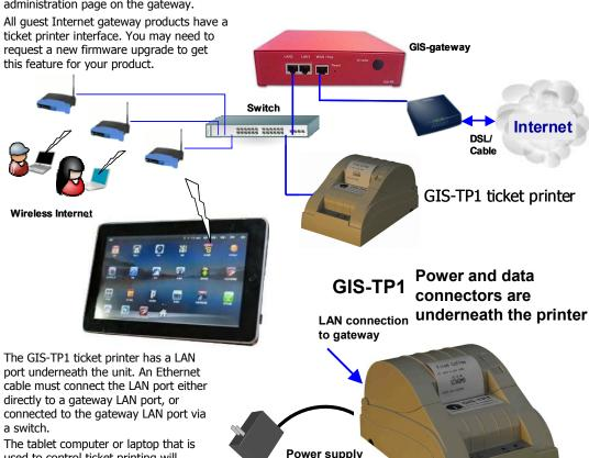
**USE ONLY THE 12volt, 3amp POWER SUPPLY SHIPPED** WITH THE GIS-TP1 UNIT TO PREVENT DAMAGE
