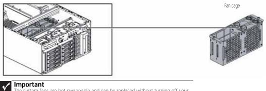
The system fans are hot-swappable and can be replaced without turning off your server.
