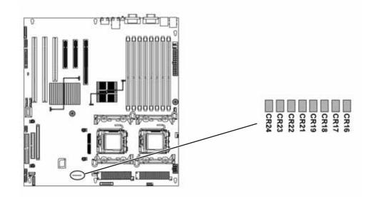
The eight diagnostic LEDs are divided into two groups. LEDs from CR16-CR19 comprise one group, and LEDs from CR20-CR24 comprise the other group. The two groups represent the two digits of the hex code. The CR16-CR19 group stands for the first digit and the CR20-CR24 group stands for the second.
