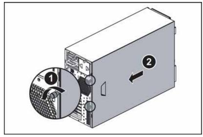
7 Slide the cover (2) toward the back of the case, then remove it from the case.
