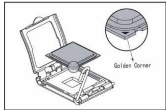
9 When the processor is oriented correctly and in place, press it firmly into the socket, rotate the load plate into place, and push down the load lever until it clicks into place.
