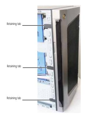
6 Swing the bezel out 45° from the front of the case, then disengage the tabs on the right side of the bezel from the chassis and remove it.
