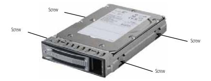
3 Using the four screws you removed, install the new hard drive into the drive tray.
