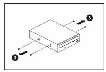
7 Install the four screws (1) you removed in the previous step on the sides of the new optical drive.
