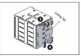
10 Remove the backplane and place it in a static-free bag for storage.
