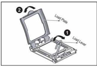
7 Lift the processor (3) out of the socket and place it in a static-free bag or case for storage.
