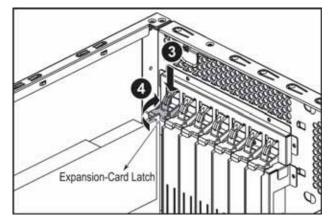
5 Gently remove the PCI card from the card slot, then lift the PCI card out of the chassis.
