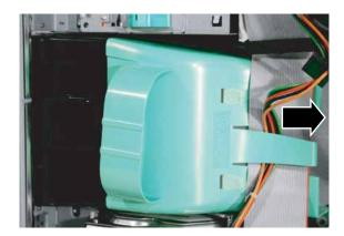
4 Grasp the air duct handle and remove the processor air duct from the chassis.
