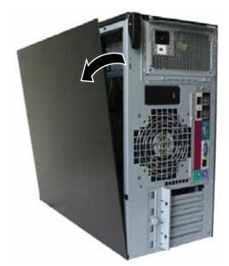
6 Lift the panel away from the server and place it out of the way.
