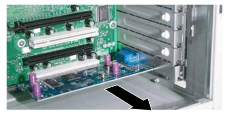
**6** Press the new card into the expansion slot. To help insert the card you can slightly rock the card end-to-end, but do not bend the card sideways.
