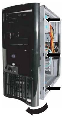
3 Swing the right side of the bezel out until the left side of the bezel can be disengaged from the left side of the computer, then remove the bezel.
