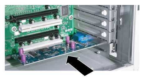
7 Swing the card retention bar back into place and tighten the captive thumbscrew.
