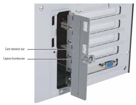
If you are replacing a card, remove the old expansion card. To loosen the card you can slightly rock the card end-to-end, but do not bend the card sideways.
