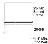
Allow minimum clearances for freezer door and fresh food door for a full 130° door swing and to allow for pan removal.
