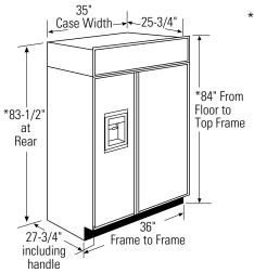
\* Shipping height. The refrigerator can be adjusted to fit into a cutout that is 83-1/2" min. to 84-1/2" max. height. Note that the top case trim at the front is 1/2" higher and will overlap upper cabinetry or soffit. Use leveling legs and wheels for a maximum 1" height adjustment.
