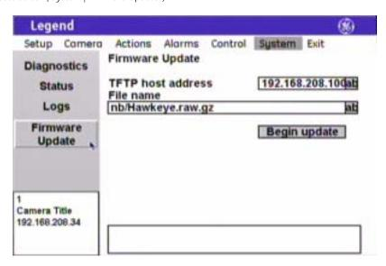
To update (or reload) the dome's software using the Firmware Update feature, see *Figure 54* and do the following:
