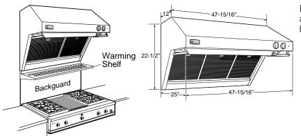
Each hood is shipped with a stainless steel backguard and a warming shelf. Hoods may be installed with the shelf or backguard alone, or with both as shown.
