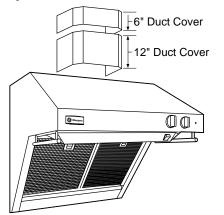
Decorative duct covers are available in 6" and 12" heights. Duct covers may be stacked, in various combinations, to conceal the ductwork running from the top of the hood to the ceiling.
