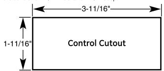
We recommend that the cutout in granite or other hard surfaces be made before the countertop is installed.
