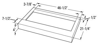
A stainless steel liner is shipped with each hood insert. This non-combustible liner protects the underside of the canopy. **Custom Liner**
