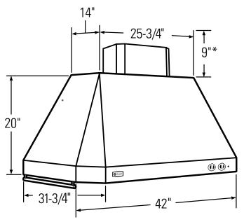
\*9" for ceiling heights of 7' 11" to 8' 5" using the supplied support frame and duct cover.
