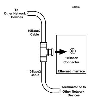
Connecting the CMM742 Ethernet Interface to a 10Base2 Network with "T" Connector
