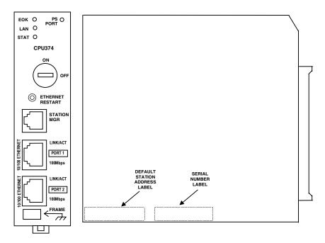
IC693CPU374 Series 90-30 CPU Module with Ethernet Interface
