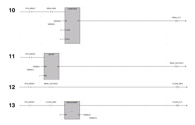
**Rung # 10**: The COMMREQ Function Block has three input parameters and one output parameter.
