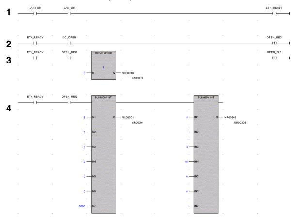
**Rung # 1**: Input LANIFOK (bit 16 of the LAN Interface Status bits) monitors the health of the Ethernet Interface. Input LAN\_OK (bit 13 of the LAN Interface Status bits) monitors the online/offline status of the Ethernet Interface. If both bits are set it is OK to send a COMMREQ and the ETH\_READY coil is ON. ETH\_READY is used as an interlock for Rungs 2-16.
