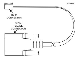
If your terminal or PC is unable to communicate with the Ethernet Interface through the RS-232 port, consult the documentation for your terminal or PC to verify that your connection is wired correctly.
