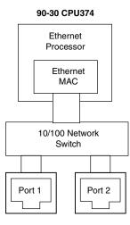
For simple installations, the embedded switch allows PLCs and other devices to be connected together without requiring any additional components.
