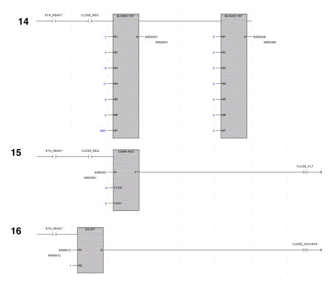
**Rung # 14**: The BLKMV INT functions set up the COMMREQ Command Block contents. When this rung is activated, the constant operands are moved into the memory beginning at the address indicated in the instruction. The constant operands in this example are defined in the Close Modbus/TCP Connection Example in this chapter.
