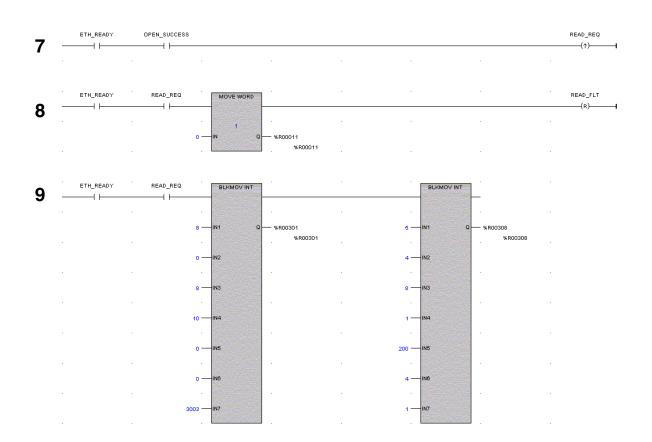
**Rung # 7**: When OPEN\_SUCCESS is set it triggers READ\_REQ, which enables execution of the BLKMOV, MOVE and COMMREQ functions for the Modbus/TCP Read Commreq. READ\_REQ is a one-shot (Positive Transition) coil, activating once when OPEN\_SUCCESS transitions from OFF to ON.
