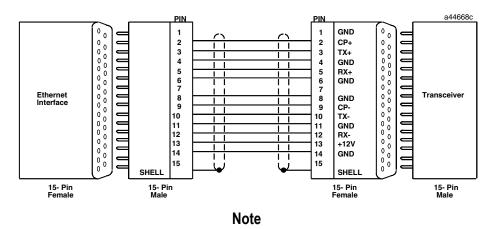
Pinouts are provided for troubleshooting purposes only. Cables are readily available from commercial distributors. GE Fanuc recommends purchasing rather than making transceiver cables.
