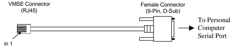
Figure 6-10. VMSE to VersaMax Serial Cable
