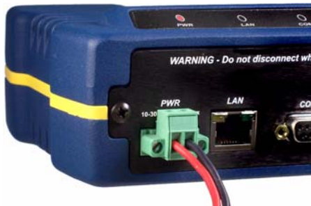
Figure 2. Power Connector (Polarity: Left +, Right –)
