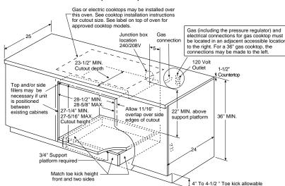
Optional Undercounter Installation With 30" CleanDesign or Sealed Burner Gas Cooktop (in inches)
