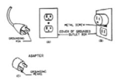
installed by a qualified electrician. The green colored rigid ear, lug, or the like extending from the adapter must be connected to a permanent ground such as a properly grounded outlet box cover. Whenever the adapter is used, it must be held in place by a metal screw.
