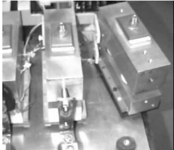
Figure 21. Removing the SCR Module from the mounting plate..
