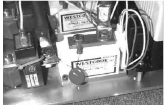
Figure 14. Location of SCRs on size M, Z, N ASTAT-IBP.
