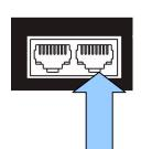
The RJ45 end connects to the outside receptacle of Port 1 of the PB3 unit and the DB9 end connects to your PC's COM Port (typically COM1).
