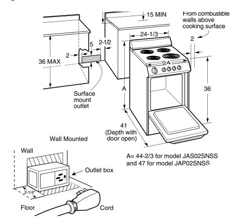
Recommended acceptable electrical outlet area. Orient the electrical receptacle so the length is parallel to the floor.
