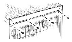
Take out four screws at the top rear of the cabinet, lift the top slightly at the rear and push it forward to remove it.
