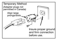
**CAUTION:** Attaching an adapter ground terminal to the wall outlet cover screw does not ground the appliance unless the cover screw is metal, and not insulated, and the wall outlet is grounded through the house wiring. You should have the circuit checked by a qualified electrician to make sure the outlet is properly grounded.
