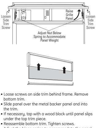
• Adjust the hinge spring to accommodate the panel weight, if necessary.
