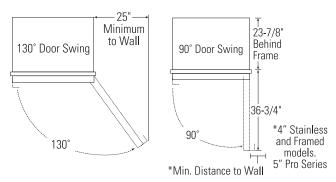
Allow 25" minimum clearance for a full 130° door swing. Allow 15" for pan removal.
