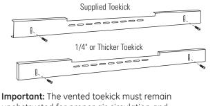
unobstructed for proper air circulation and refrigerator operation.
