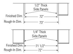
Note: 1/2" thick side panels shown. Side panels can be any thickness. Add side panel thickness to outside trim width (36" or 72" for two models) to calculate the rough-in dimension. The leading (front) edge must be finished to match surrounding cabinetry.
