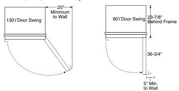
Allow 25" minimum clearance for a full 130° door swing. Allow 15" for pan removal. for a 90° door swing, allow 5" minimum clearance for professional models. If the 90° doorstop position is used, pan access is maintained but pan removal is restricted.
