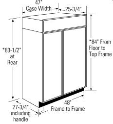
\* Shipping height. The refrigerator can be adjusted to fit into a cutout that is 83-1/2" min. to 84-1/2" max. height. Note that the top case trim at the front is 1/2" higher and will overlap upper cabinetry or soffit. Use leveling legs and wheels for a maximum 1" height adjustment.
