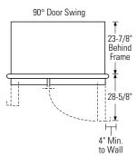
Allow minimum clearances for freezer door and fresh food door for a full 130° door swing and to allow for pan removal.
