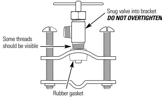
*Optional water supply connection (using saddle valve)\**
