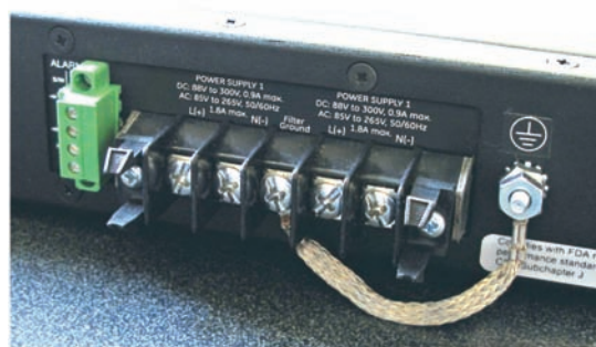
FIGURE 7: Power connection and alarm contacts
