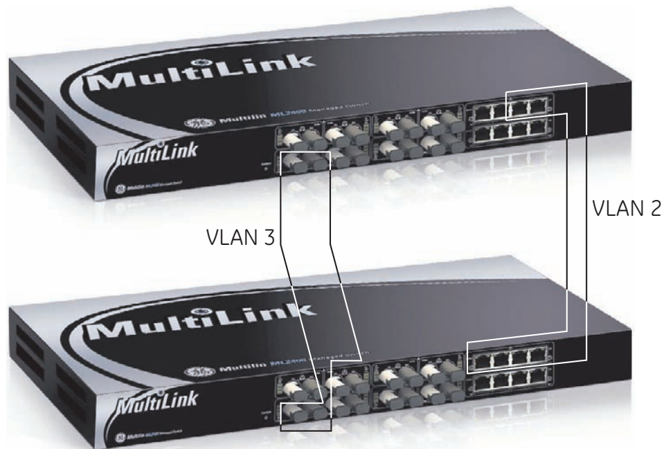
FIGURE 15: Tagged Virtual LANs
