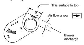
When the blower is in position, snap the blower retainer bar toward the front into the indent. Reattach the plug into the junction box.
