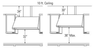
10 ft. Ceilings: Install the hood 32" min. to 36" max. above the cooking surface. The duct cover will expand to a maximum of 34" above the top of the hood to meet the ceiling.
