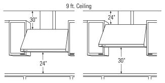
**9 ft. Ceilings:** Install the hood 24" min. and up to a maximum of 30" above the cooking surface. The duct cover will expand to reach ceiling height.
