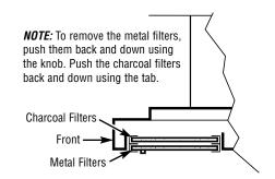
For proper operation, be sure to use the charcoal filters in the upper set of filter holders and metal filters in the lower set of filter holders.
