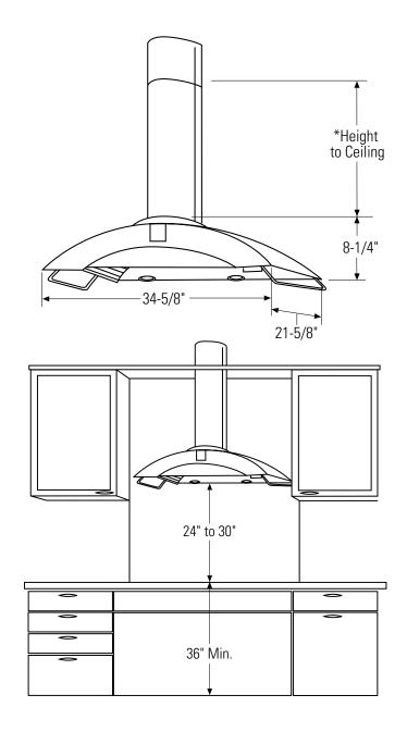
The vent hood must be installed 24" min. and 30" max. above the cooking surface depending on the ceiling height.
