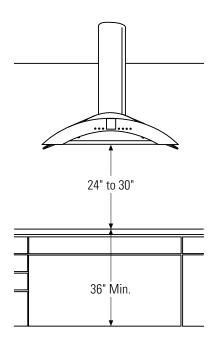
The exact installation height is determined by the ceiling height and duct cover trim strips provided with the hood. For optimum performance, the hood must be installed 24" min. and 30" max. above the cooking surface.
