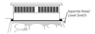
All 36" models are equipped with a separate raise/lower switch. The switch must be installed in a separate location outside of the vent and cooktop cutout.
